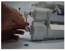
Step 2. Insert collet tool onto tubing, hold tubing by fingers, push collet tool up in order to remove broken fitting part
