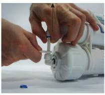
Step 2. Insert collet tool onto tubing, hold tubing by fingers, push collet tool down in order to remove broken fitting part
