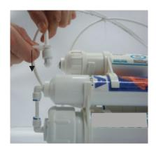
Step 2. Disconnect broken fitting from tubing. Hold tubing with one hand, insert collet tool into tubing and press collet tool down.
