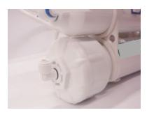
Step 5. Screw new fitting onto head
