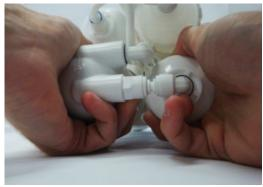
Step 5. Direct tubing onto fitting, and press together membrane housing and 4th stage filter
