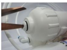
Step 3. Unscrew (counter clockwise) broken fitting using pliers. Some fitting broken down at the base, and there it is hard to grab rest of fitting by pliers You can use scissors instead (picture below).
