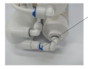
Step 1. Remove 2 of blue C-rings from the broken fitting
