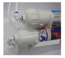
Step 1. Remove blue C-ring from the broken fitting
