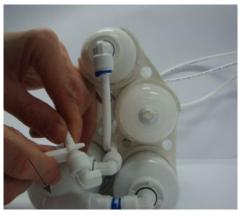
Step 2. Remove broken piece of fitting. Hold tubing, insert collet tool onto tubing, push collet tool down pressing fitting.
