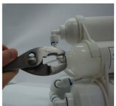
Step 3. Remove broken fitting from opening. Use pliers or scissors (check page #2)
