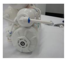
Step 3. Turn fitting counter clockwise for 90 degree (you can easy reach to broken fitting area)
