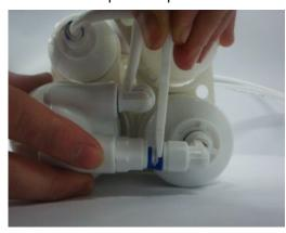
Step 2. Insert collet tool between both fittings and push it right as shown on picture. Disconnect broken part from tubing
