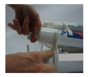
Step 5. Lift one side of second stage filter aprox 1" up. You can hold membrane housing by another hand
