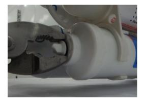
Step 3. Use pliers or scissors to remove second part of broken fitting
