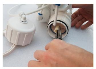
Using pliers remove old membrane. Remove new membrane from the plastic bag. Try not to touch the membrane with fingers. Insert new membrane the same side as old membrane was
